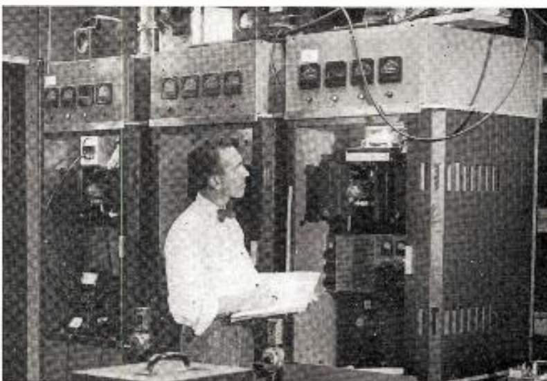
FINAL test of an RCA Victor uhf transmitter is being made preparatory to shipment. The transmitter shown, including video, audio and control units, was one of the first four shipped from Camden last Friday.
